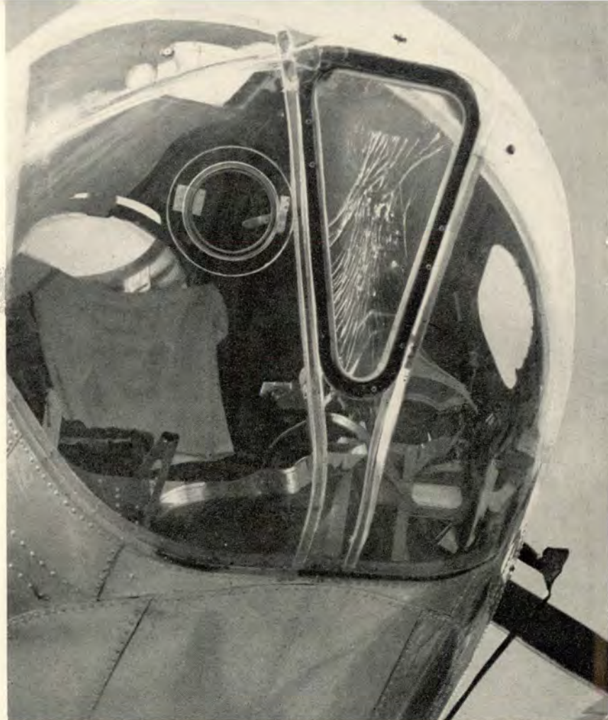
A terrific jolt of lightning damaged the nose of this B-17. The center section is bulletproof glass. All antennas were burned off.
