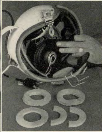
Foam rubber pads insure comfort; eliminate most external noises.
