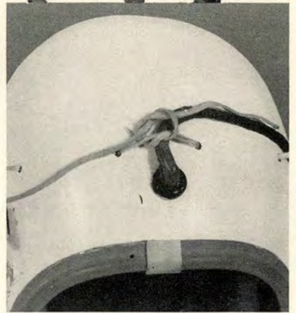
After tightening, lacing should be secured around cord with a square knot.
