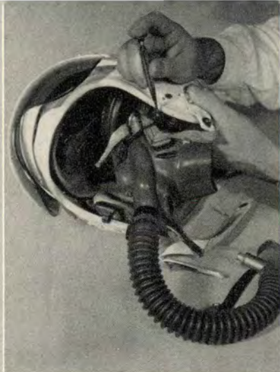
Oxygen mask should be attached to the helmet by brass machine screws.
