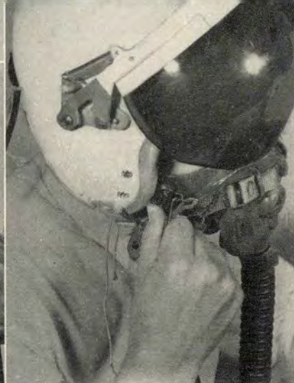
This is proper grip for removing mask. The clasp works easily after you practice a few times.
