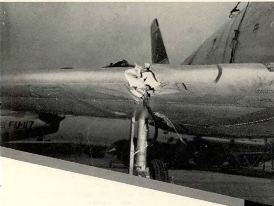
While most lightning strikes are made on slow-moving aircraft, fighters aren't immune as this picture of an F-86 will show (above). Lightning strikes a C-47, damaging the left aileron (right) and burning the static eliminator.
