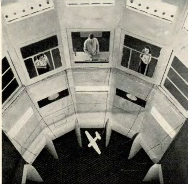
Before actual spin tests are made, experts run lab checks on various single-engine aircraft design configurations.
