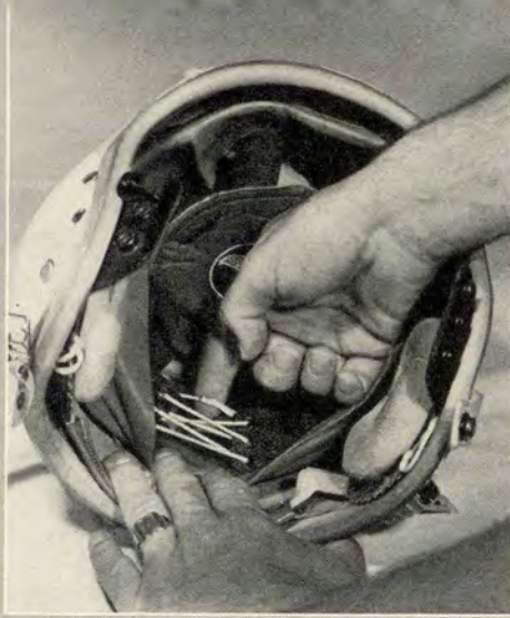
Headband should be taken up slowly, trying on helmet after each change.
