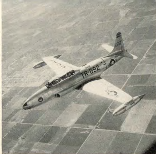
According to factory test pilots, proper spin recovery can only be effected when the tip tanks are empty.
